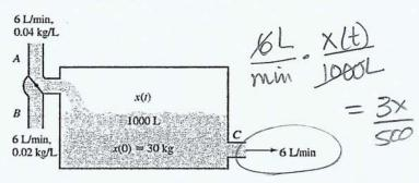
Initially, 30 kg of salt is dissolved in the tank which has a volume of 1000 L. The outlet pipe C, which empties the tank at a constant rate of 6 L/minute, maintains the contents of the tank at constant volume. Assuming the tank is kept well stirred, determine the amount of salt in the tank at time t > 0. X = aut Y salt after t minutes.
